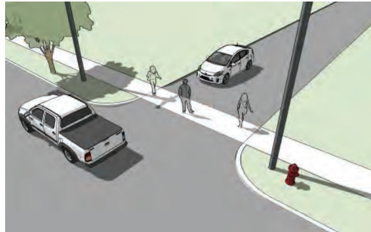
Driveways should rise up to sidewalk using the same material as the sidewalk for driveway crosswalks. The sidewalk should not drop down to the driveway.
