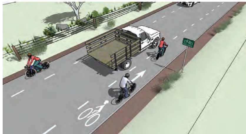
When there is no room for bicycle lanes, advisory bike lanes are more effective than sharrow markings at messaging that bicycles might be present.
