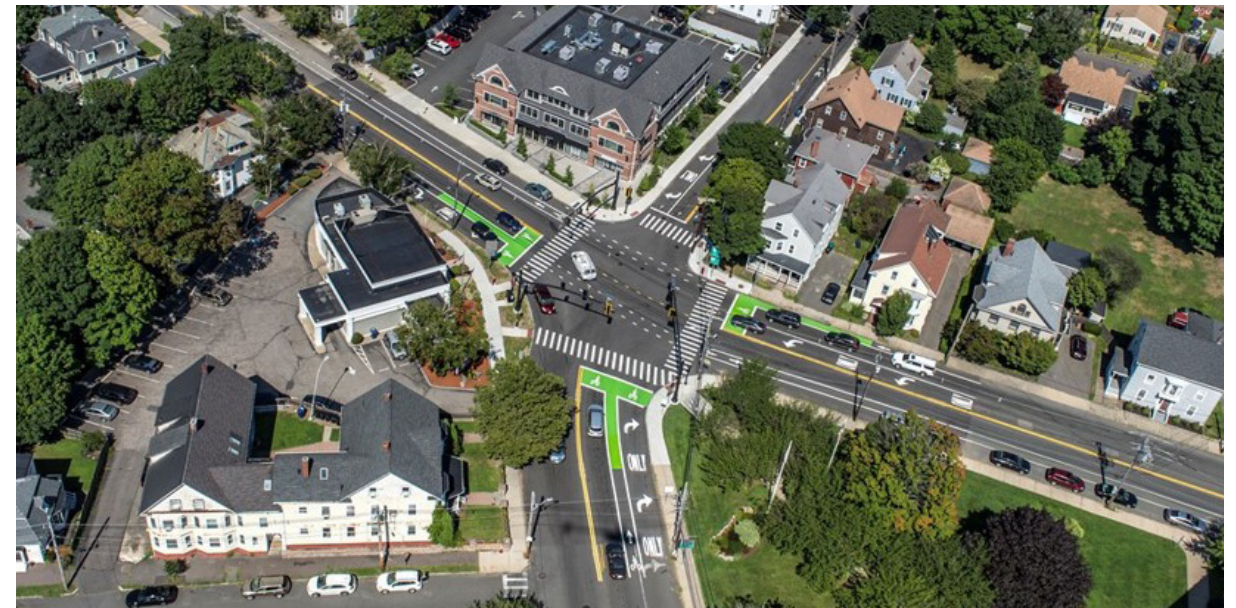
Figure 10-7. Rantoul Street in Beverly was successfully dieted for most of its length with a variety of tools, including new on-street parking, bike lanes and removal of excess lanes.
