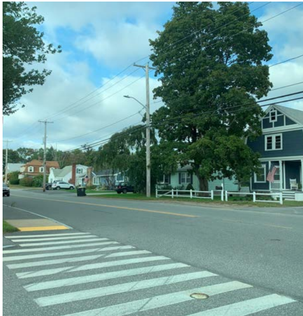
Figure 10-3. A typical crossing in the Pond Street neighborhood only carries across the minor side street with no crosswalk for the higher volume arterial. West Main Street has only six crosswalks on its entire length of nearly 1.5 miles through some of Avon’s densest neighborhoods.
