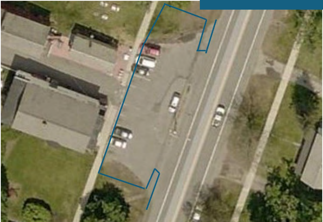
Narrow the entrance to the parking lot in front of Mim's Market and the Creamie, via curb cuts, to slow the speed of vehicles entering/exiting.
