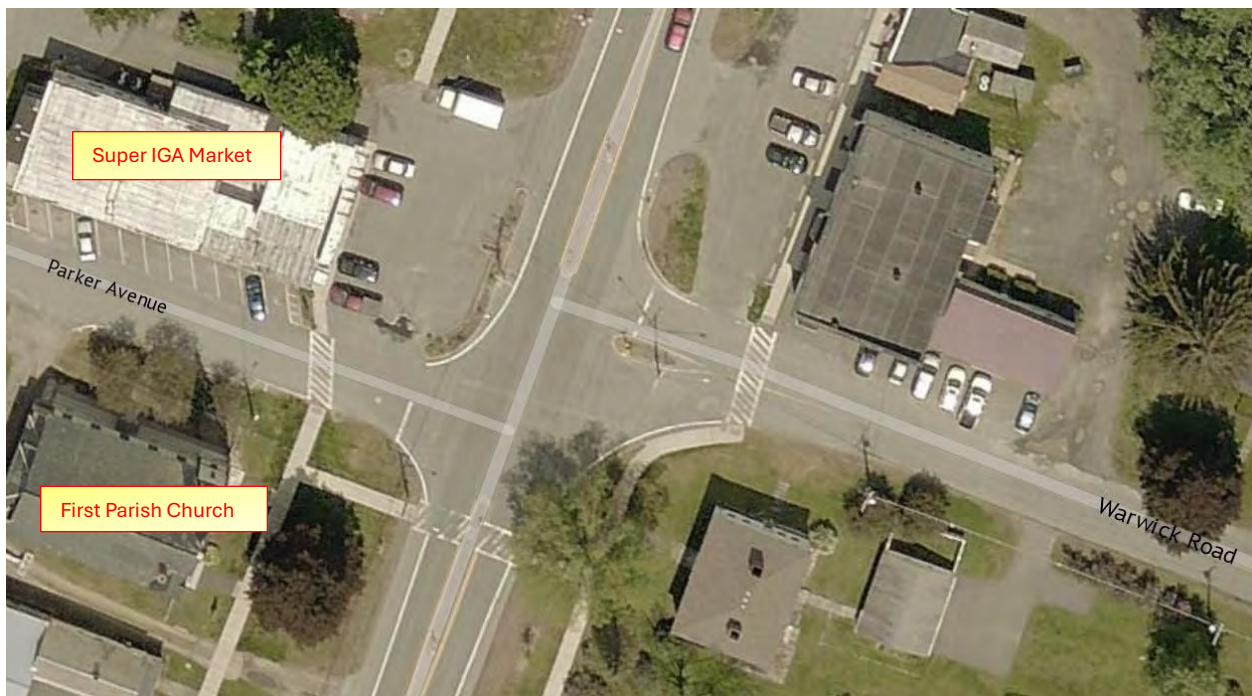
Unsafe road geometry and markings at Main/Parker/Warwick/IGA intersection (MassDOT Pictometry, Eagle View, 2017)
